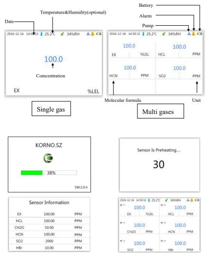
Long press the "Power" button, the screen will light up and display the sensor information. It needs about 1 minutes to warm up the gas detector. After power on, the screen will display the configured gas/ gases.
